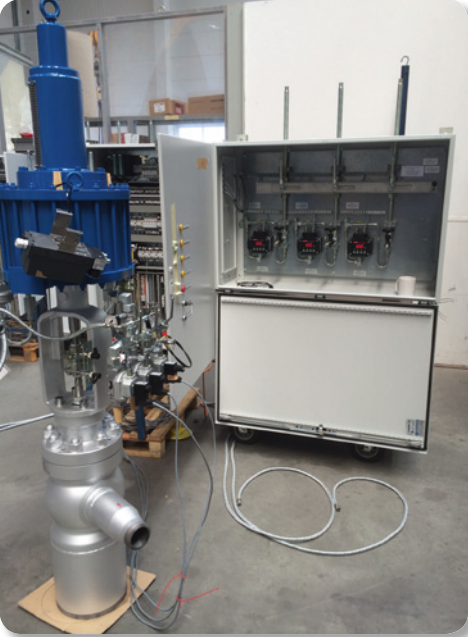
PRDS as controlled safety valve incl. component-tested steam rod
