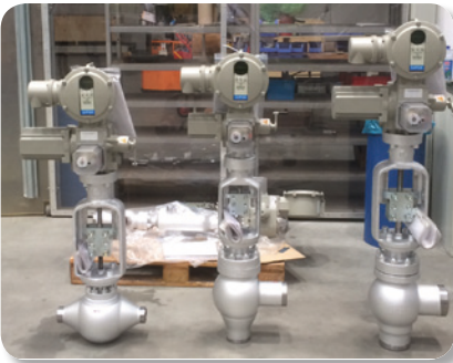
HP boiler control valves
